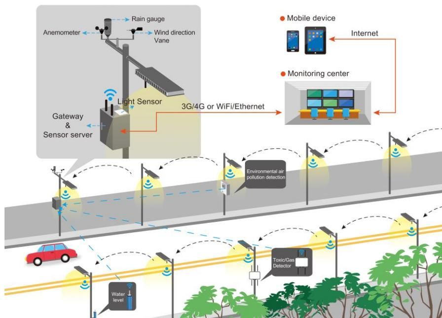
**Figure 1: Example of an intelligent streetlighting network with various sensors that communicate to the CMS and mobile devices<sup>2</sup>**
